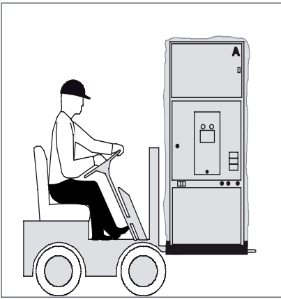
Fig. 3.4 Transport using a forklift truck
